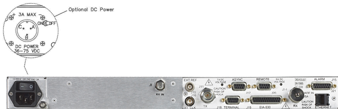
Figure 5-1. DMDVB20 LBST Satellite Modem Rear Panel Configurations
